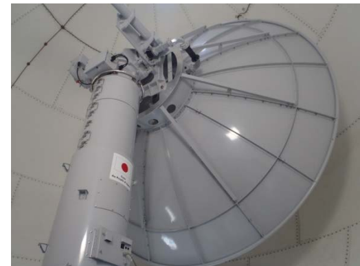
Aparri radar antenna
