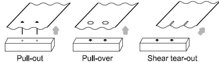
(b) Roof-column connection failure
