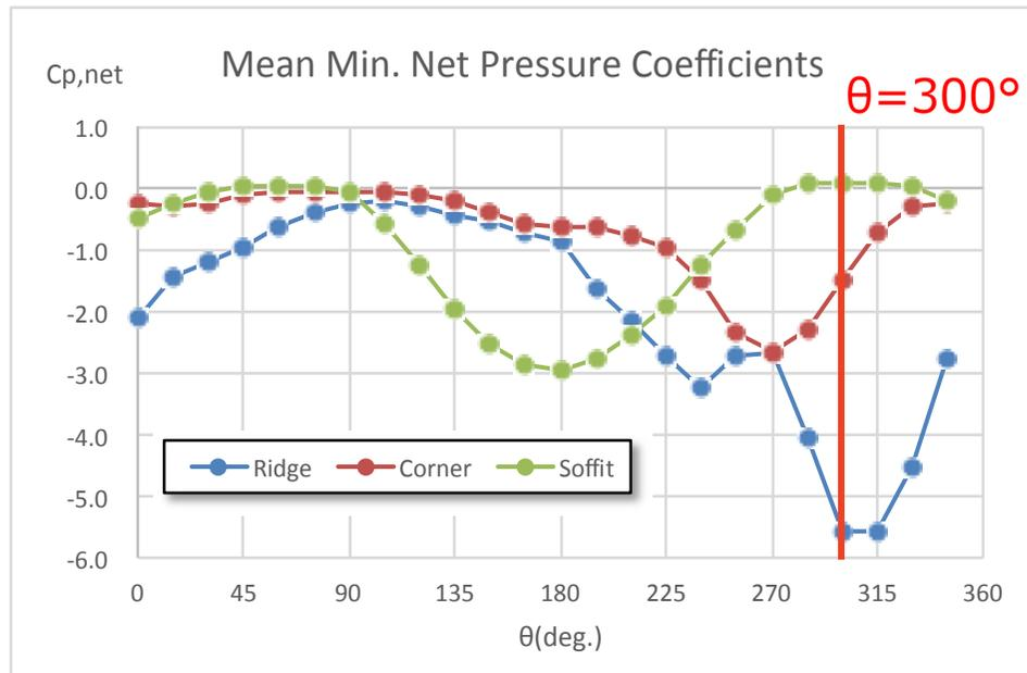
Unique characteristics of wind loading was observed, which arises due to its large openings
