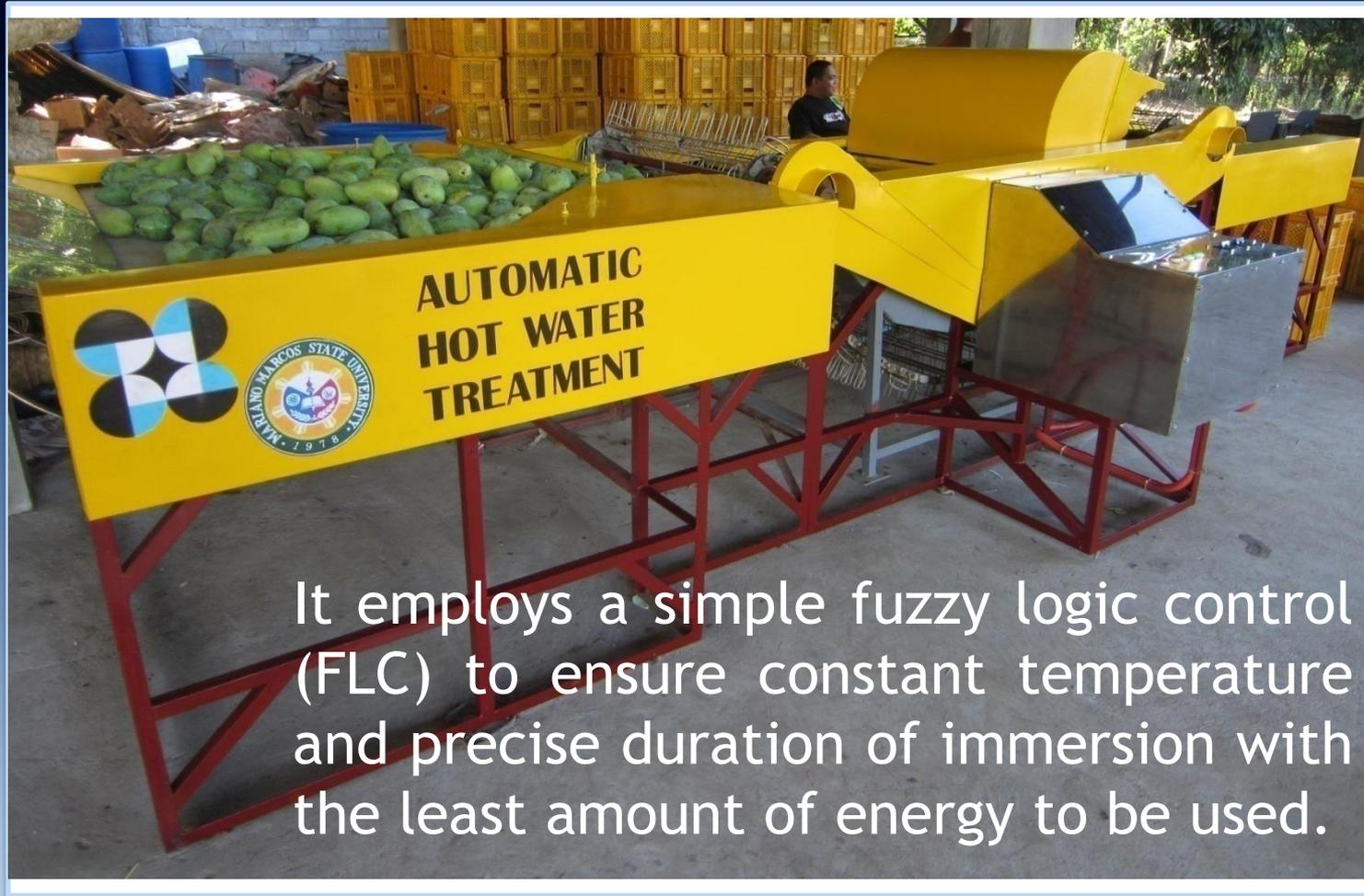
It employs a simple fuzzy logic control (FLC) to ensure constant temperature and precise duration of immersion with the least amount of energy to be used.
