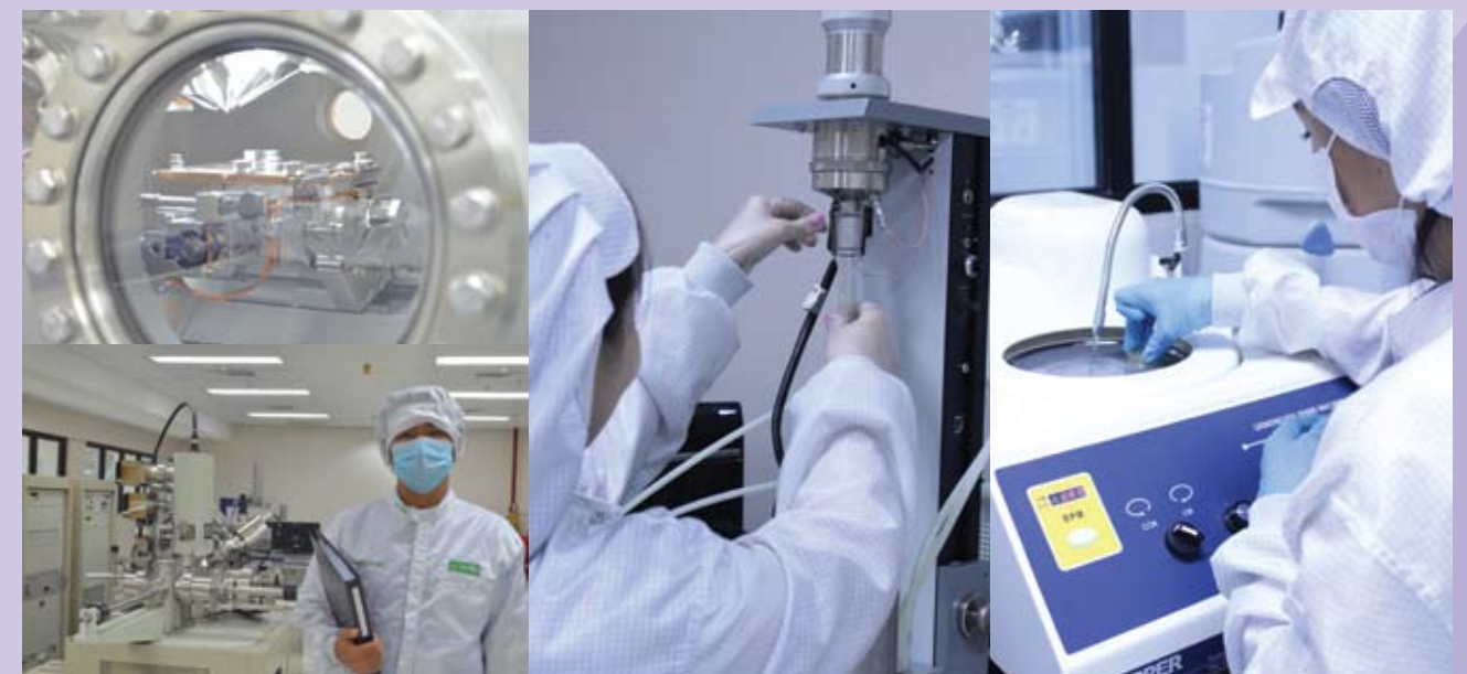
JAMP 9500F Field Emission Auger Electron Microprobe (bottom, left); A look inside the sample chamber of the Time of Flight - Secondary Ion Mass Spectroscopy (TOF-SIMS) - the sample chamber of the machine where analysis and detailed elemental and molecular information is obtained (top, left); Placing sample into the furnace of Thermo Mechanical Analyzer (TMA) to begin analysis (center); Sample preparation using polisher and grinder (right) (Images courtesy of ADMATEL)
