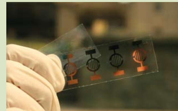
High quality metal contacts as well as a transparent conducting oxide contacts for solar cell applications (Image courtesy of Nanostructured Solar Energy Devices Program)
