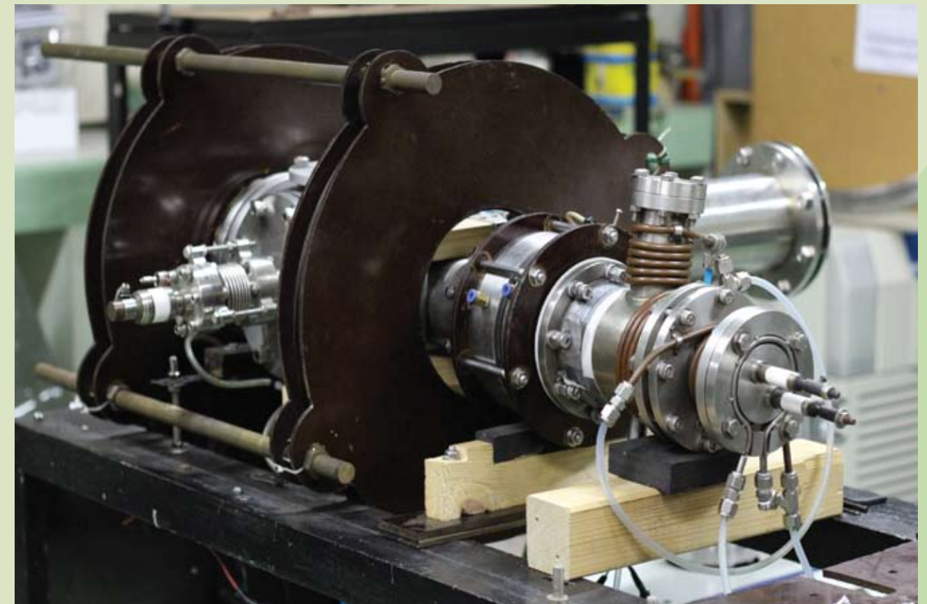
Sheet Plasma Negative Ion Source used for MAX Phase Thin Film Deposition (Image courtesy of the Advanced MAX Phase Project Team)
