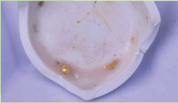
Gold bead recovered using the CHLORIDE-HYPOCHLORITE LEACHING STAGED PRECIPITATION PROCESS (Image courtesy of MinERS Project A)
