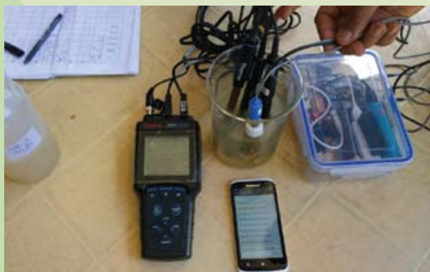
Ateneo Sensor Control box with plug-ins for pH, conductivity, DO communicates wirelessly with Android phone. (Image courtesy of Chemical Sensors Project 5)
