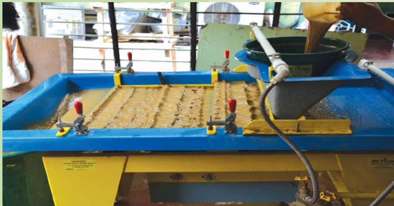
Micron mill wave table used to concentrate low-grade ore samples (Image courtesy of S&T Responsible Mining in Mindanao Project 8)
