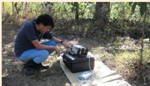
Field measurement of radon gas in soil using alpha GUARD PQ2000 PRO radon monitor (Images courtesy of Radon Project Team)
