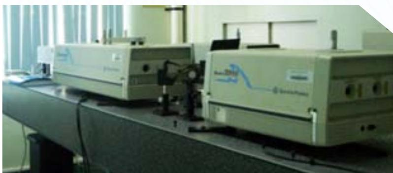
*In 2011, PCIEERD supported the laboratory upgrading of the National Institute of Physics (NIP) of the University of the Philippines Diliman. Through the funding assistance, NIP will upgrade its femtosecond laser facility to be able to perform terahertz time-domain spectroscopy. Shown in the photo are the current femtosecond laser and frequency doubler at NIP.*
