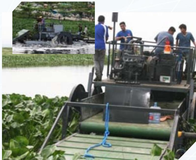
A group of technicians from the Metro Manila Development Authority tested the harvester at a swamp near the Taguig Pumping Station. The harvester was developed to collect free-floating water hyacinth by cutting them onsite and conveying them to the platform hold.
