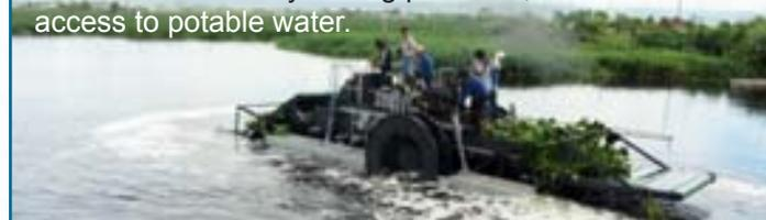
*One of DOST’s High-Impact Technology Solutions projects is the water hyacinth harvester, which was developed due to the need for the mechanical removal of water hyacinth in inland bodies of water and river systems in the country.*
