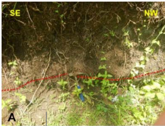
Sensor deployment site: Traces of the right lateral boundary of the moving mass
