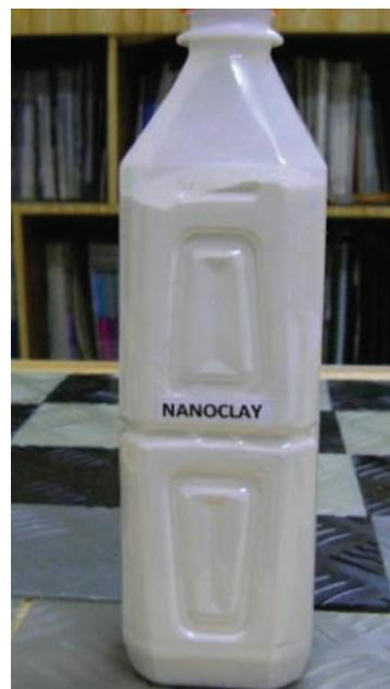
**The project “Development of Biodegradable Starch-clay Nanocomposite for Advanced Food Packaging” aims to develop biodegradable nanocomposites from local sources for advanced food packaging. Montmorillonite clay from Cebu was synthesized with a non-ionic modifying agent to make the clay compatible with thermoplastic starch.**
