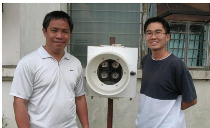
**The project “An Improved Air Pollution Sensor Utilizing Differential Optical Absorption Spectroscopy Technology” developed an instrument that measures ambient concentrations of sulfur dioxide, ozone and nitrogen dioxide. Shown in the photo are project leader Dr. James B. Simpás with research assistant Sherdon Niño Y. Uy beside the retroreflector.**
