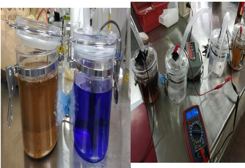
MFC containing substrate (anodic chamber) and 500ppm  $\text{Cu}^{2+}$  (cathodic chamber)
