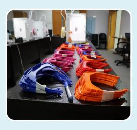
3D printing of face shield frames at the AMReL facility. Below are the outputs from this initiative.
