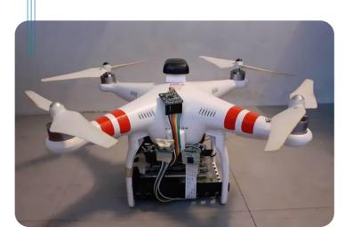
The artificial-intelligence-based (Al-based) mobile thermal scanner attached to a drone is designed to easily scan and pinpoint people with high body temperature. The drones provide real-time data transmission, equipped with a Global Positioning System (GPS), and a communication capacity within the range of 2 km. This technology is especially useful in shortening queues, minimizing contact at checkpoints, and immediately identifying individuals for monitoring.
